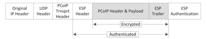
**UDP-encapsulated ESP Packet Format**
